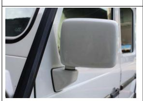
The mirror (A) 6 functions is fitted for the original W463 G class '86-'12 has CAM BUS system and the mirror with no indicator light but with electric folding and mirror glass memory system.
