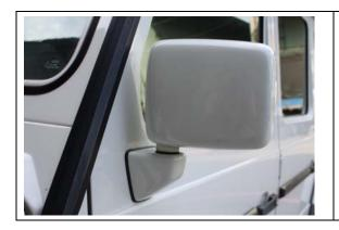
The mirror (C) 2 functions is fitted for the original W463 G class '86-'12 has no CAM BUS system and the mirror with no indicator light, no electric folding and no mirror glass memory system.
