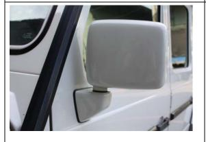
The mirror (B) 5 functions is fitted for the original W463 G class '86-'12 has no CAM BUS system and the mirror with no indicator light, no electric folding and no mirror glass memory system.
